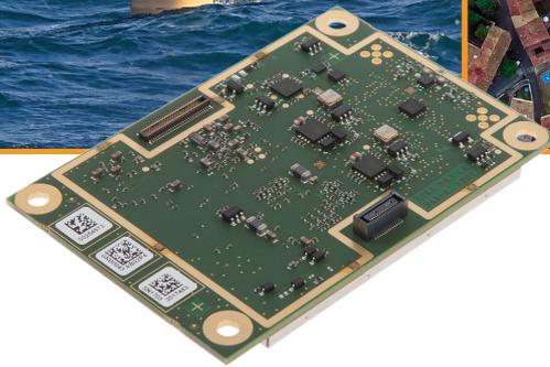
The AsteRx-m2 is a compact, high-performance, ultra-low power GNSS receiver ideal for integration in UAS, handheld devices and other demanding industrial applications where power and space are at a premium. It incorporates the latest in anti-jamming technology and offers unbeatable robustness and reliability.
